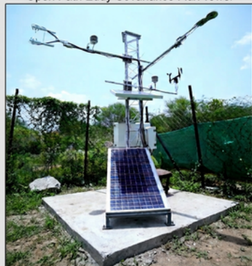
Open Path Eddy Covariance Flux Tower
