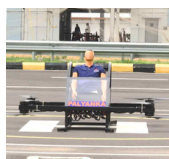
Palyanka – Medical Drone (TIHAN) A heavy-payload autonomous ambulance drone designed to transport up to 200 kg for emergency medical evacuation, disaster relief and cargo delivery in difficult terrains.
