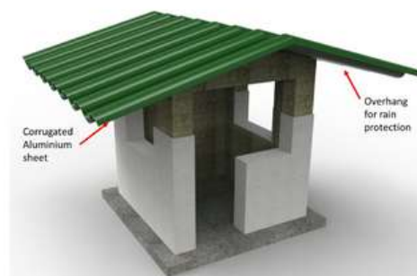
Figure 19: All side overhanging roof with corrugated aluminium sheet
