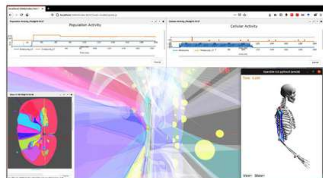
Figure 8: A screenshot from NEUROiD in silico movement platform with the spinal cord controller (centre), slice view (left) and the upper limb musculoskeletal model (right). Traces of electrical activity may be seen on the top panel.
