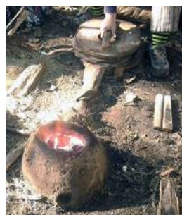
Fig 1. Iron-making experimental bowl furnace utilizing charcoal
