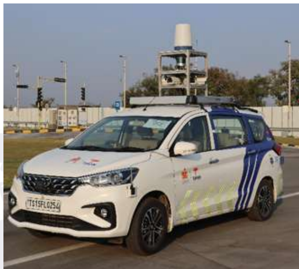
Figure 3. SAFARI – TiHAN IITH Data Collection Vehicle
