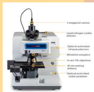
Figure 2. The RaptIR+ microscope with its different components.
