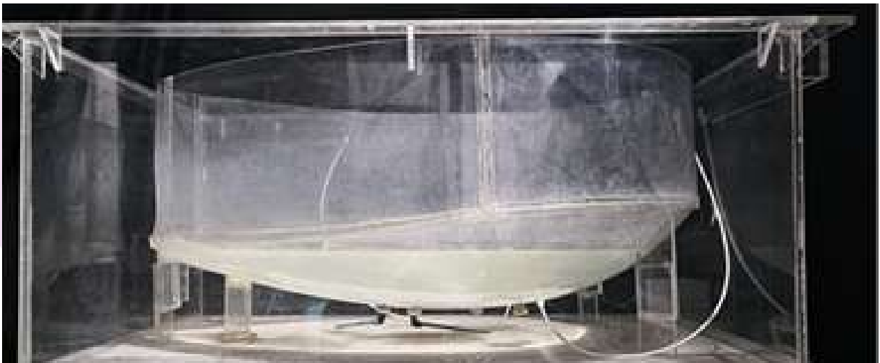
Figure 3. A scaled down cold model setup of an Industrial Electric Arc Furnace.
