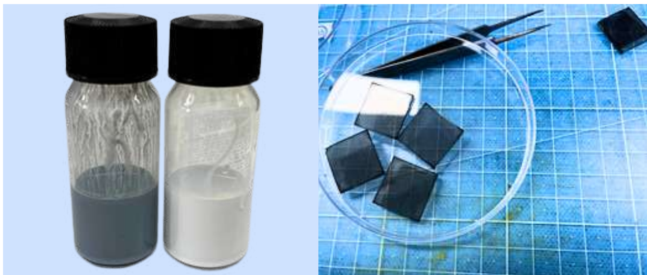
Figure-3: Solar Paint Composition (L) and Glass slides coated with Solar Paint which functions as an electrode (R)
