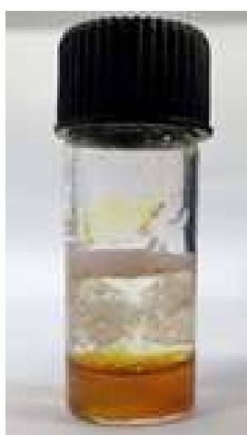
Rhodamine B dye After catalytic degradation by AgNPs
