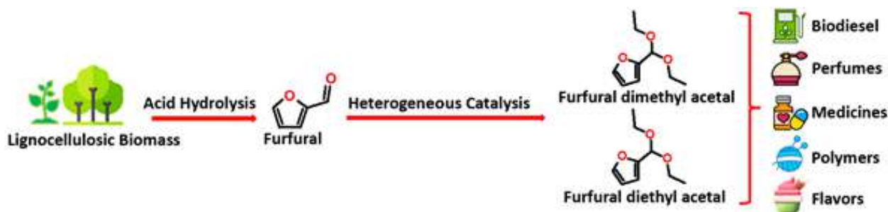
Figure-1: Catalytic route for the production of furfural dialkyl acetals from biomass derived furfural
