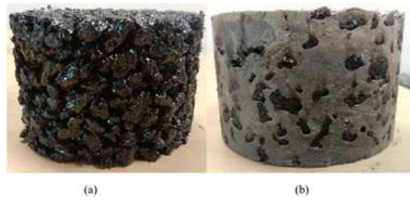
Figure 2 (a) Porous asphalt mixture containing 50% RAP material; (b) Cement grouted bituminous mixtures containing 50% RAP material
