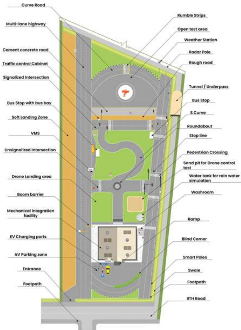
Figure-2: Plan of Connected Autonomous Vehicle Testbed at IITH
