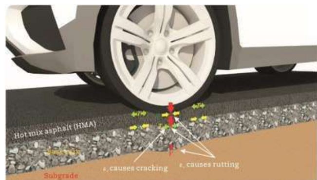
Impact of AVs on Pavement Structure due to platooning
