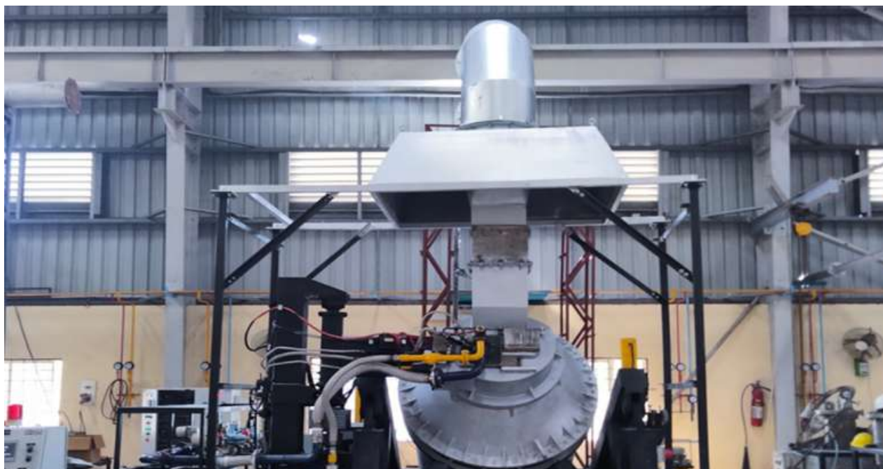
Fig. 2a): Rotary tilting furnace for PCB recycling
