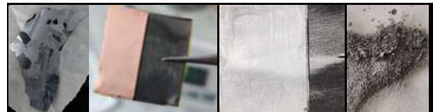
Fig. 2: Recovered metals from EOL solar PVs. In the Combinatorial Materials Lab, MSME, IITH
