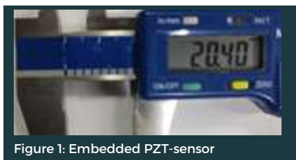
Figure 3: Embedded PZT sensors for continuous monitoring after casting and during service life of structure
