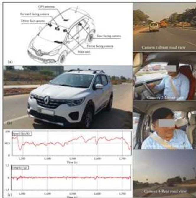
Figure 13: (a) Instrumentation details; (b) Study vehicle; (c) Recorded speed and acceleration profiles; and (d) snapshots of collected video data.
