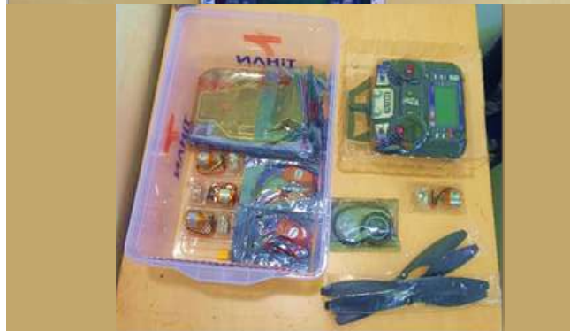
Figure 9: UAV kit developed for skill development
