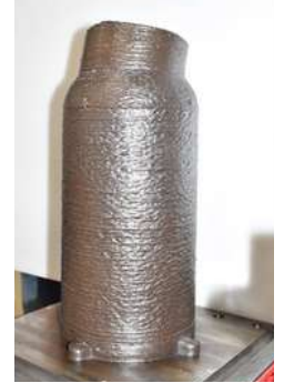
Figure - Complete deposited Part of Motor casing
