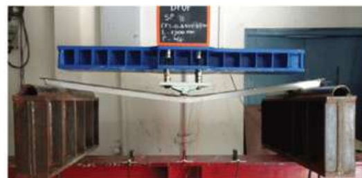
Figure Caption: Development of Light weight flooring system
