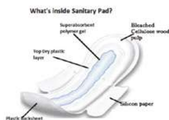
Figure Caption: Different layers of a typical sanitary pad (Source: www.scienceandsamosa.com )
