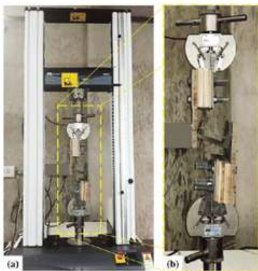
Figure Caption: Newly developed test setup to determine the stiffness of the sheathing boards in the wall panel
