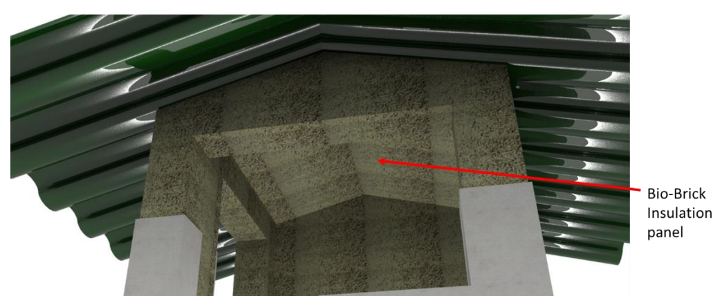
Figure 5: All side overhanging roof with corrugated aluminium sheet
