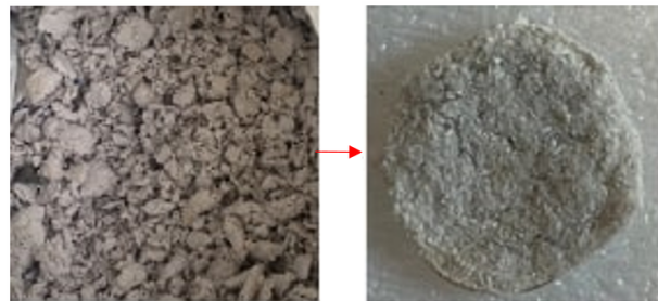
Fig. 1: Conversion of paper sludge to foam
