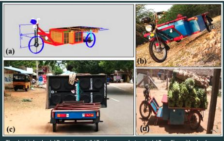
The electric loader. (a) Design layout, (b) Testing on rocky terrain, (c) Travelling with a load on a rural road, (d) Transporting agricultural produce to the local market
