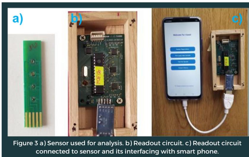
Figure 3 a) Sensor used for analysis. b) Readout circuit. c) Readout circuit connected to sensor and its interfacing with smart phone.
