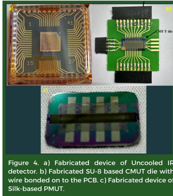
Figure 4. a) Fabricated device of Uncooled IR detector. b) Fabricated SU-8 based CMUT die with wire bonded on to the PCB. c) Fabricated device of Silk-based PMUT.
