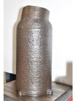
**Figure - Complete deposited Part of Motor casing**
